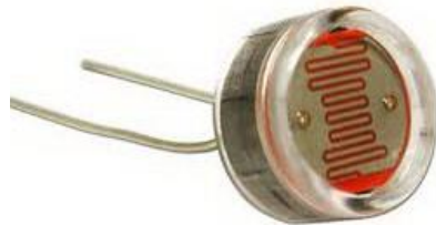
Gambar 2.21 LDR ( Light Depending Resistor )
