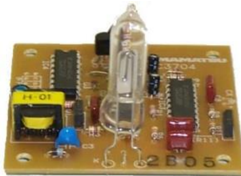
Gambar 2.25 Modul sensor cahaya ultraviolet UVtron
