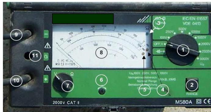
Gambar 2.31 Alat Ukur Megaohm Meter <sup>2</sup>
