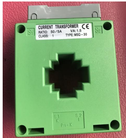
Gambar 3.2 CT (Current Transformer) Pertama
