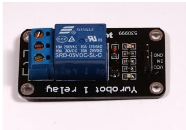
**Gambar 2.22 Modul Relay 1 Channel**
