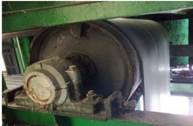
Gambar 2.5 *Bend Pulley*
