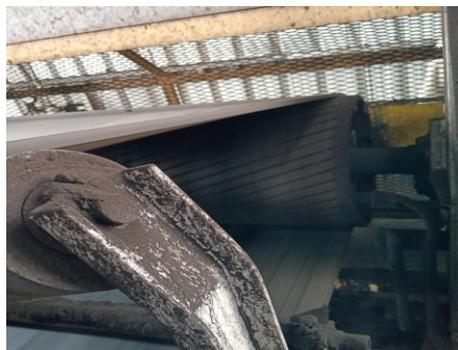
Gambar 2.6 *Head Pulley*
