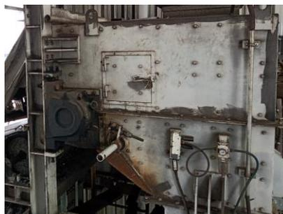
Gambar 2.15 Block Chute Switch
