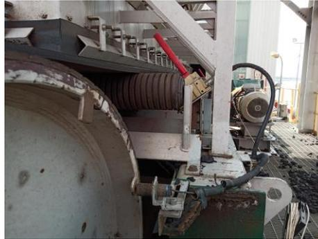
Gambar 2.16 Zero/Low Speed Switch
