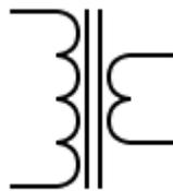
**Gambar 2.14** Simbol Transformator Step-Down (Putra, 2017)
