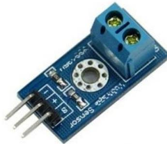
**Gambar 2.20** Modul sensor tegangan (Saptaji, 2016)
