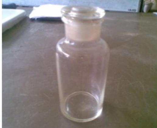
**Gambar 4. Alat Piknometer**
