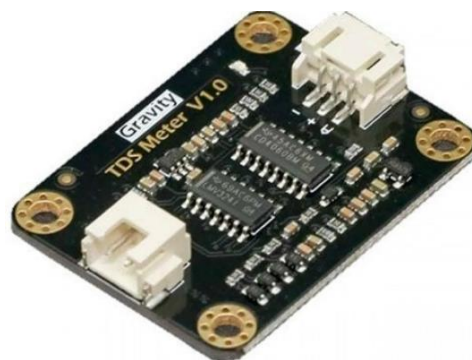
Gambar 2.4 TDS Meter Analog (dfrobot, 2018)
