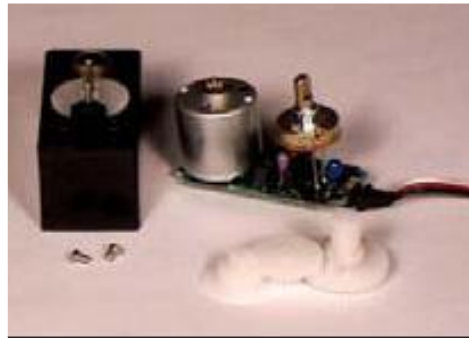
Gambar 2.9 Sistem Mekanik Motor Servo
