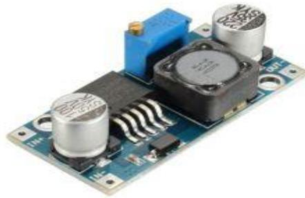
**Gambar 2.5** DC Converter LM2596 [14]
