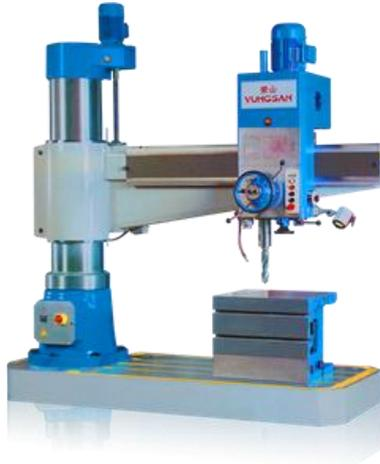
Gambar 2.20 Mesin Bor Radial
