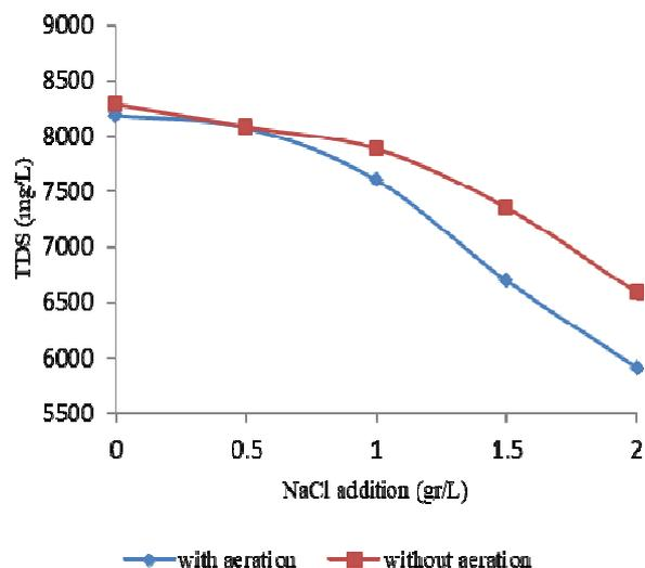
Fig. 3 Effect of aeration processes and NaCl concentration on TDS
