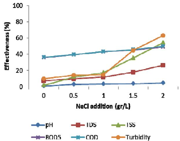
Fig. 9 Electrocoagulation effectiveness of NaCl addition without combination aeration processes
