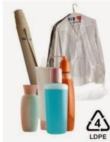
Gambar 2.1 Plastik LDPE (*Low-Density Polyethylene*)
