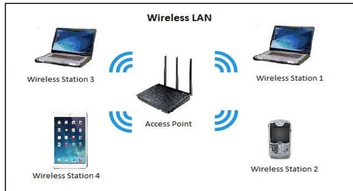
**Gambar 2.4** Model WLAN
