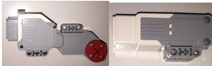
**Gambar 2.5** (a) *Large Motor* ; (b) *Medium Motor*
