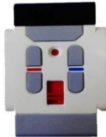
**Gambar 2.16** *Remote Infrared Beacon*
