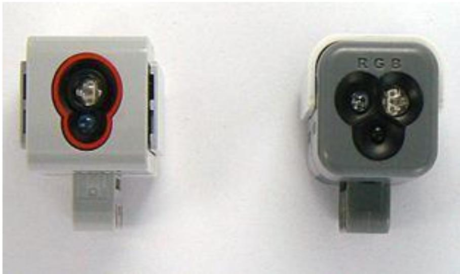
**Gambar 2.10** Sensor Warna (*Colour Sensor*)
