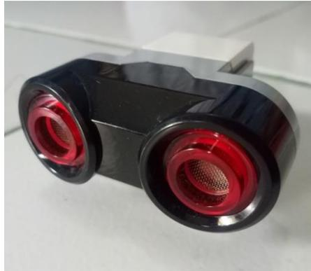
**Gambar 2.12** Sensor Ultrasonik
