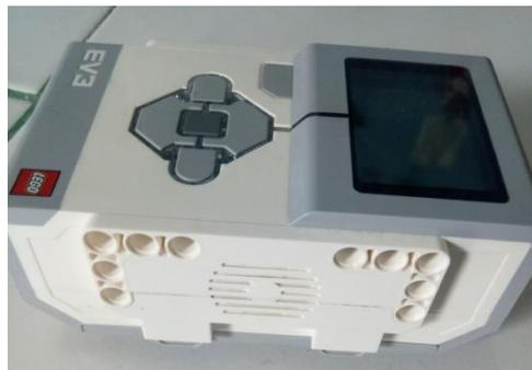
**Gambar 2.8** EV3 *Intelligent Brick* Bagian Kanan
