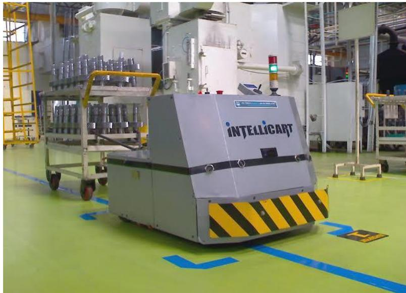
**Gambar 2.2** Robot Intellicart – *Towing AGV(Automatic Guided Vehicles)*
