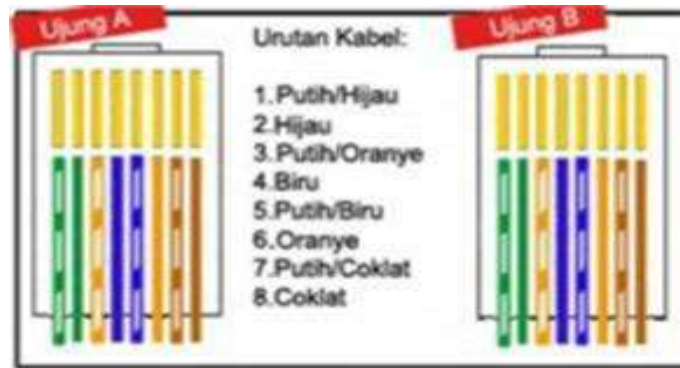
Gambar 2.12. Pemasangan kabel straight through T568B
