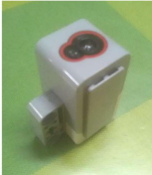
**Gambar 2.21** Sensor Warna Mindstorms EV3
