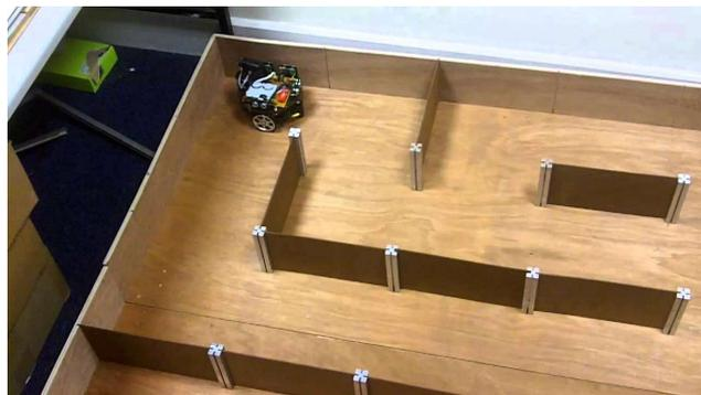
**Gambar 2.31** Robot penghindar dinding
