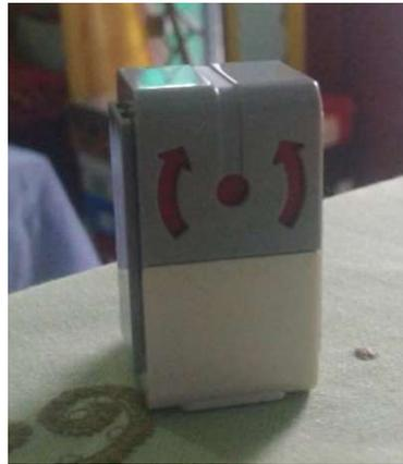
**Gambar 2.23** Sensor Gyro Mindstorms EV3
