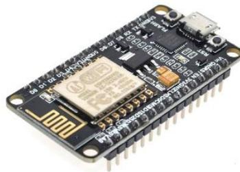
**Gambar 2.1** Modul NodeMCU ESP8266-12E
