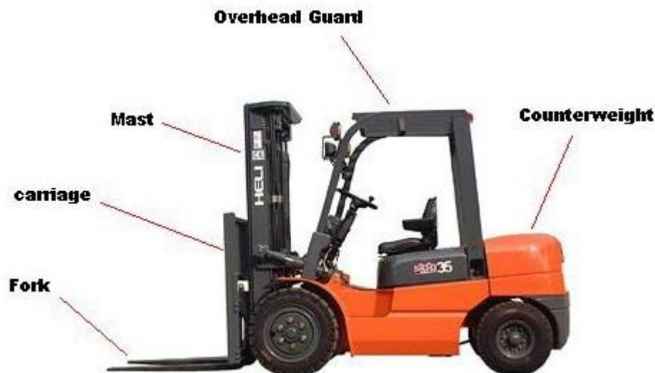
**Gambar 2.2** Bagian – bagian *forklift*
