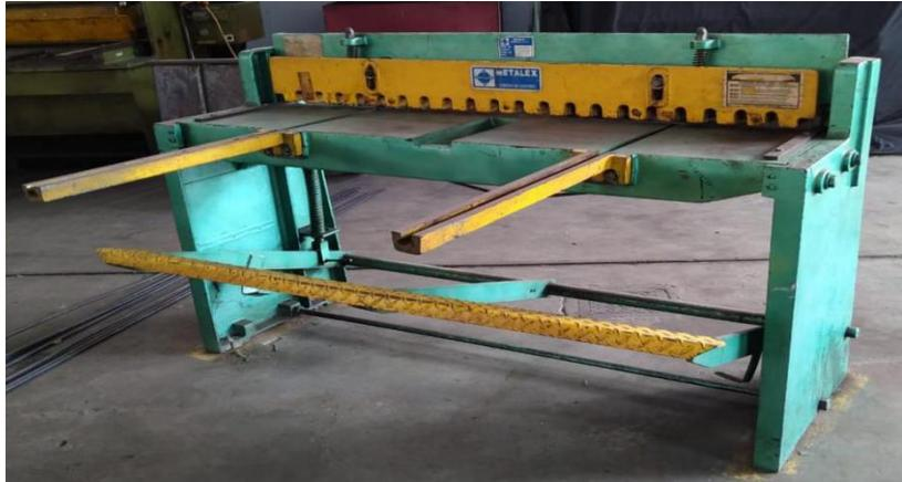
**Gambar 2.3 Mesin Gullotine Manual**
