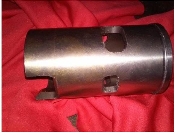
**Gambar 2.11** *Cylinder Liner*
