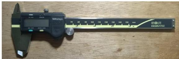
**Gambar 2.6** Mitutoyo Vernier Caliper
