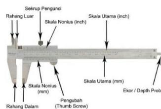
**Gambar 2.7** Bagian-bagian Jangka Sorong [8]
