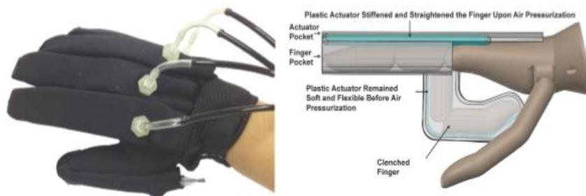
**Gambar 2.6** *Design of a Soft Robotic Glove for Hand Rehabilitation of Stroke Patients With Clenched Fist Deformity Using Inflatable Plastic Actuators* [17]
