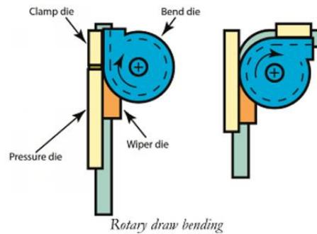
Gambar 2.2.2 *Bending Rotary Draw*
