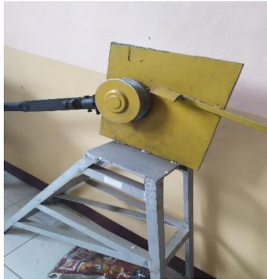
Gambar 2.2.1 Mesin *Bending* Pipa Manual
