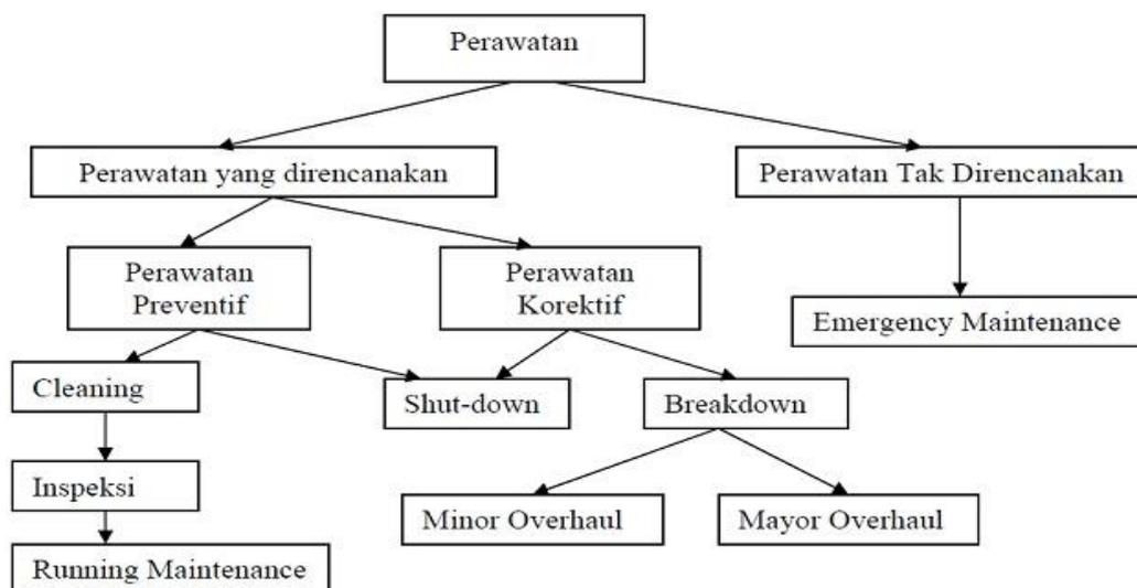
**Gambar 2.9** Diagram *Maintenance*<sup>1</sup>
