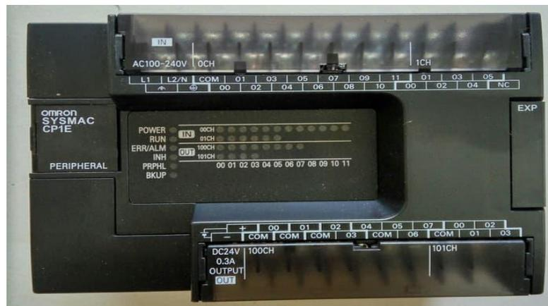
Gambar 2.1 PLC (*Programmable Logic Controller*)
