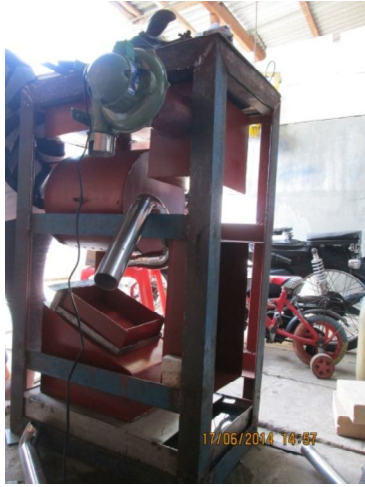
Perangkaian Secondary Chamber
