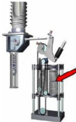
Gambar 2.17 Sistem Pegas Gulung ( Scroll )
