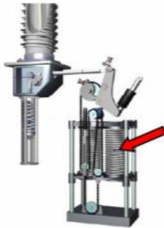
Gambar 2.16 Sistem Pegas Pilin (Helical)
