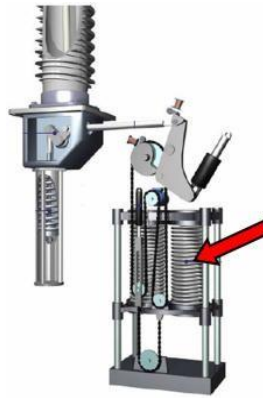
Gambar 2.13 Sistem Pegas Pilin ( Helical )
