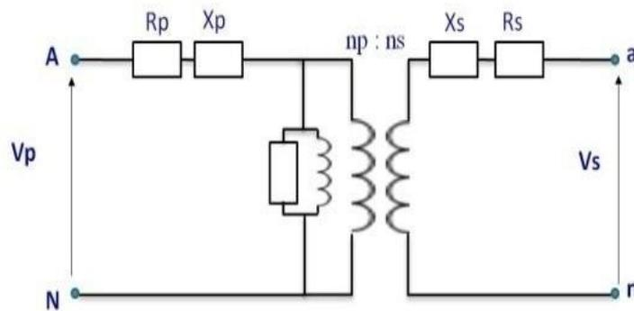
**Gambar 2.1.** Rangkain Ekivalen Transformator.
