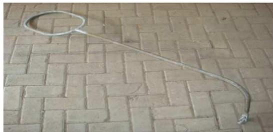
Gambar 2.40 *Arcing horn* sisi tower
