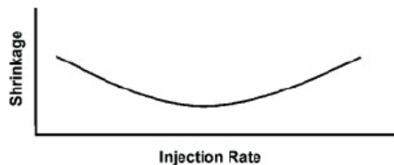
Fig. 11 The relationship between injection rate and shrinkage [19]
