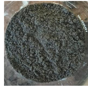
Gambar 2.3 Abu Boiler Bahan Bakar Cangkang dan Fiber Kelapa Sawit
