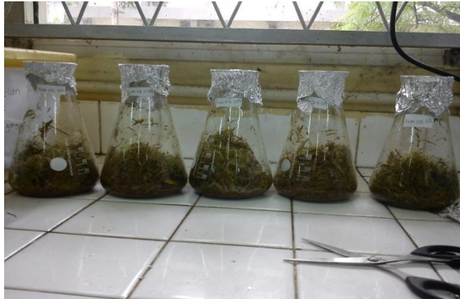
Gambar 16. Penambahan 50 ml \text{HNO}_3 5%
