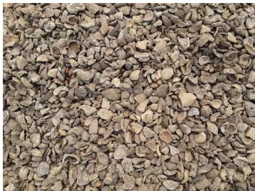
**Gambar 1. Cangkang Kelapa Sawit (PT SMS, 2014)**
