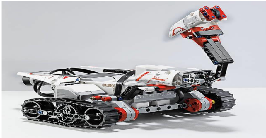
Gambar 2.1 Robot Lego Mindstroms EV3
