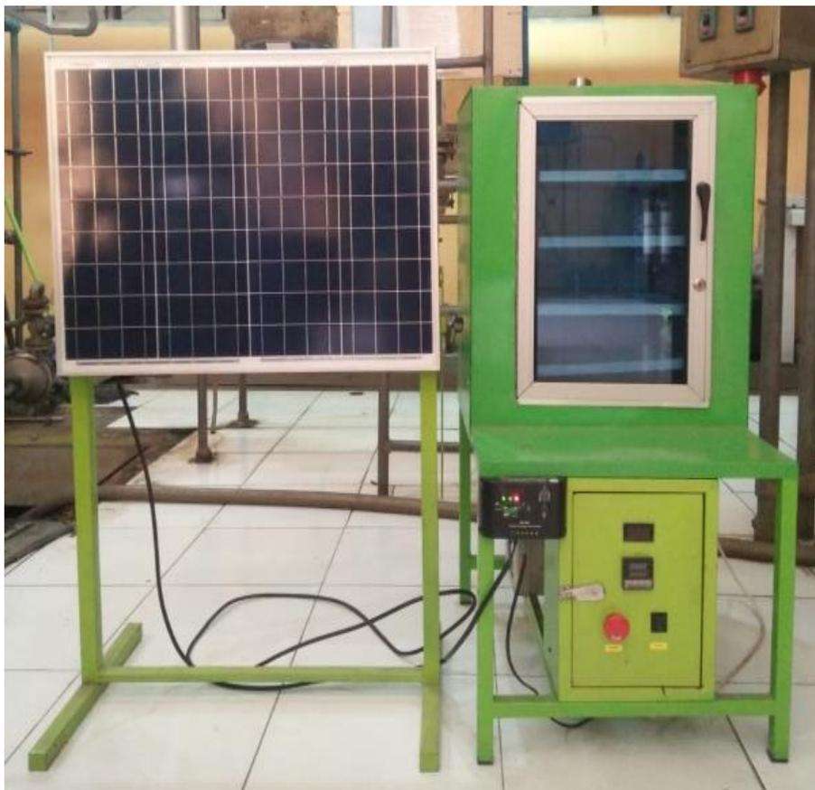
Gambar 2.4 Alat *Photovoltaic Tray Dryer*
