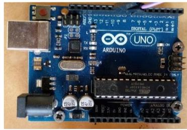
**Gambar 2.7** Board Arduino Uno (Sumber : Rean Handiko2020)
