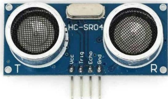
**Gambar 2.2** Sensor Ultrasonik
