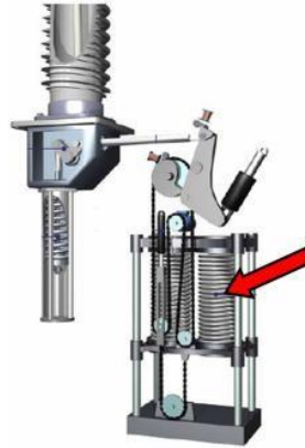
Gambar 2.13 Sistem Pegas Pilin (Helical)
