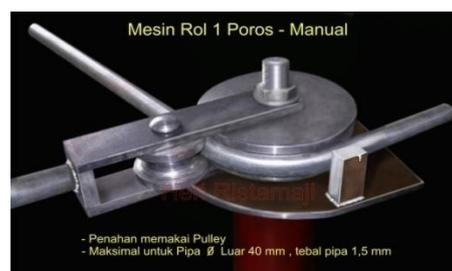
**Gambar 2.6 Alat *Bending* Pipa Manual**
