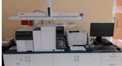
Gambar 2.1 Alat Uji GC-MS
