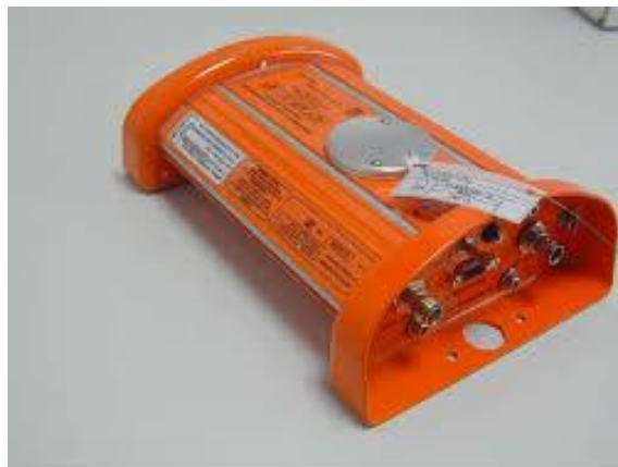
FCCID label location on ELT model ADT 496 AF-AP
