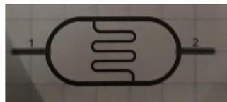
Gambar 2.5 Sensor LDR (*Light Dependent Resistor*)
