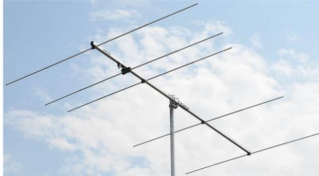
**Gambar 2.4** Antena Yagi [10]
